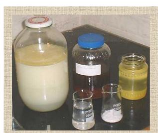
ingredients and by-products: clockwise from left - wash-water, glycerine, finished biodiesel, potassium hydroxide, methanol
