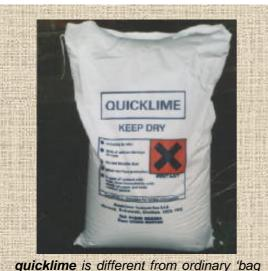
**quicklime** is different from ordinary 'bag lime' that you buy from a builder's merchants. It is calcium carbonate (limestone or chalk) which is burnt, driving off CO<sub>2</sub> to leave calcium oxide.
