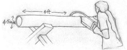
then use a hacksaw or angle grinder to cut the metal pipe into about 4ft lengths, shorter ones are possible, but make access to the 'cuffs' easier.
